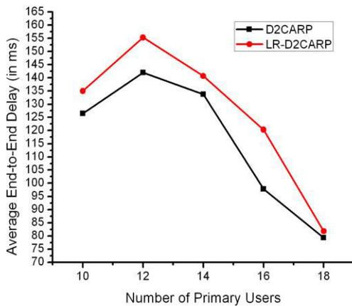
Fig. 10 Average End-to-End Delay (in ms) of D2CARP & LR-D2CARP
