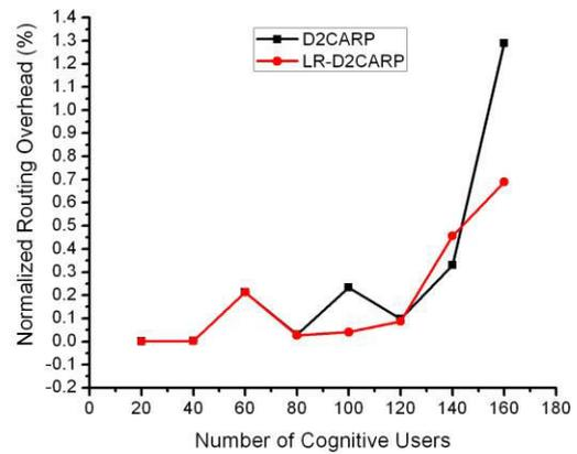
Fig. 6 Normalized Routing Overhead (in %) of D2CARP & LR-D2CARP
