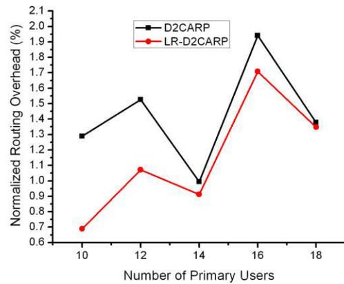
Fig. 12 Normalized Routing Overhead (in %) of D2CARP & LR-D2CARP
