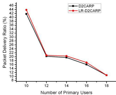
Fig. 15 Packet Delivery Ratio (%) of D2CARP & LR-D2CARP
